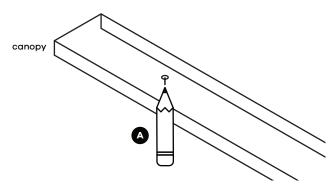
A Turn the canopy over and use the outer holes to mark the positions of the dowels.
