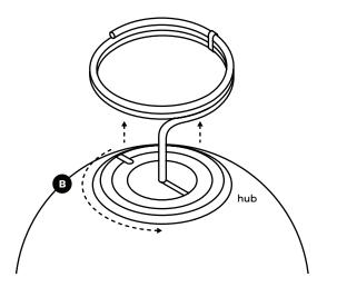
B Carefully take the lampshades out of the box with two hands. Separate the shades from the cables before assembly. For this, hold the shades with one hand and gently twist off the hub with the other hand. You can easily redock the shades later.
