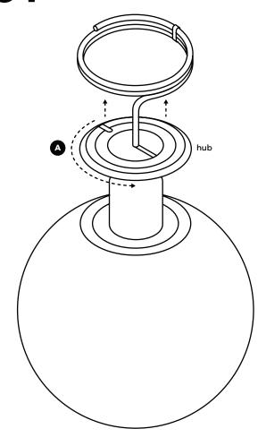
A Carefully take the lampshades out of the box with two hands. Separate the shades from the cables before assembly. For this, hold the shades with one hand and gently twist off the hub with the other hand. You can easily redock the shades later.
